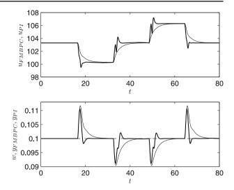
The obtained simulation results have shown that better performance criteria are obtained in the case of the FMBPC control in both control modes: the trajectory tracking mode and the disturbance rejection mode. This is obvious because the PI controller assumes linear process dynamics, while the FMBPC controller takes into account the plant nonlinearity through the fuzzy model of the plant. The proposed approach is very easy to implement and gives a high control performance.
